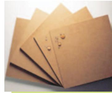
MDF is an abbreviation for medium density fibreboard. It is a type of hardboard made from wood fibres glued under intense heat and pressure. This building material is frequently sold in 4-foot by 8-foot sheets and comes in varying thicknesses similar to plywood. MDF is a common material used in many interior building projects also available in different sizes and colours in laminated and plain.
